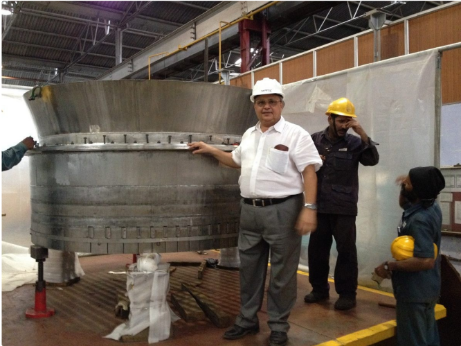
ASME Section IX Certified Inconel 800HT Nitric Acid Catalyst Basket Assembly at INOX Clean Station 2.
